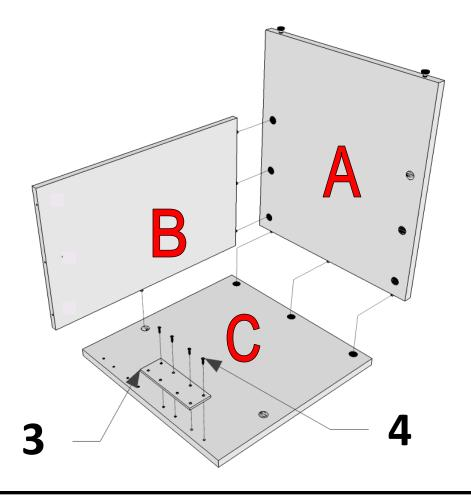
ALIGN SIDE (A) WITH MODESTY (B), PUSH TOGETHER AND TIGHTENING SCREW IN CAMS
