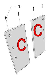
ALIGN SIDES (C)WITH MODESTY (A&B), PUSH IN PLACE AND TIGHTEN TIGHTENING SCREWS IN CAMS ITEM 5
