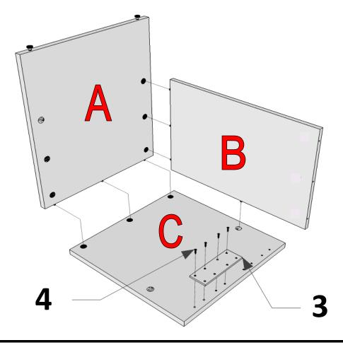
ALIGN SIDE (A) WITH MODESTY (B), PUSH TOGETHER AND TIGHTENING SCREW IN CAMS
