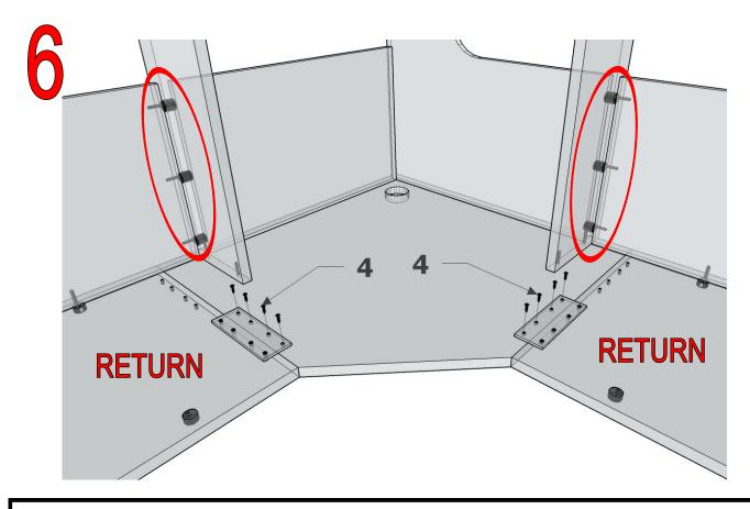
ALIGN ASSEMBLED RETURN WITH CENTRAL WORKSTATION, PINS FACING TOWARDS CIRCULAR CAMS, PUSH IN PLACE AND TIGHTEN TIGHTENING SCREW UNTIL SECURE. HIGHLIGHTED IN CIRCLES
