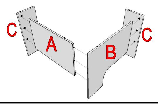
ALIGN ASSEMBLED ABOVE COMPONENTS OVER THE TOP (D) ENSURING PINS LINE UP WITH CAMS
